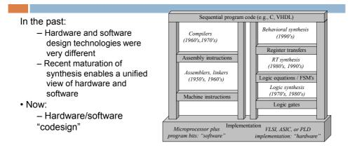
The choice of hardware versus software for a particular function is simply a tradeoff among various design metrics. there is no fundamental difference between what hardware or software can implement
